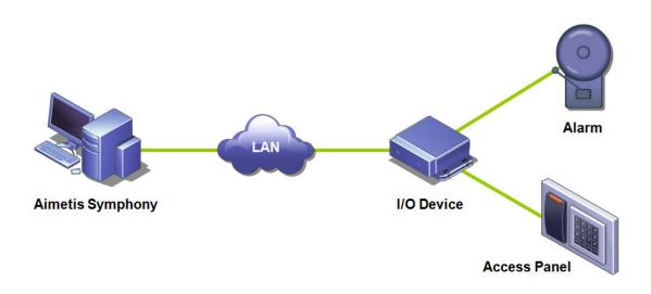
Figure 3. PC sends a signal through the LAN. The I/O device on the LAN receives the signal and then is wired to an alarm in one input or an alarm panel in another input.
