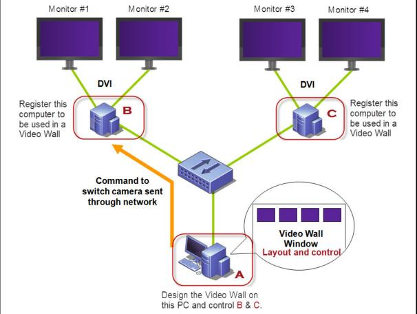
Figure 39. Video Wall setup diagram
