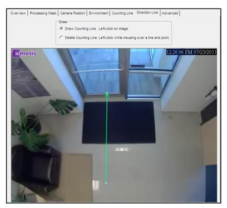
Figure 23. Direction Line subtab
