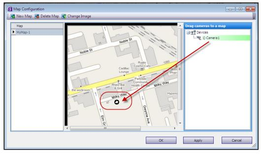
Figure 18. Drag cameras onto the map
