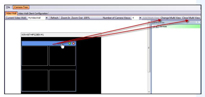
Figure 48. Activate the Change Multi View and Close Multi View buttons
