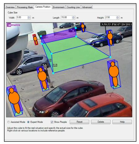
Figure 21. Virtual cube fits correctly in scene
