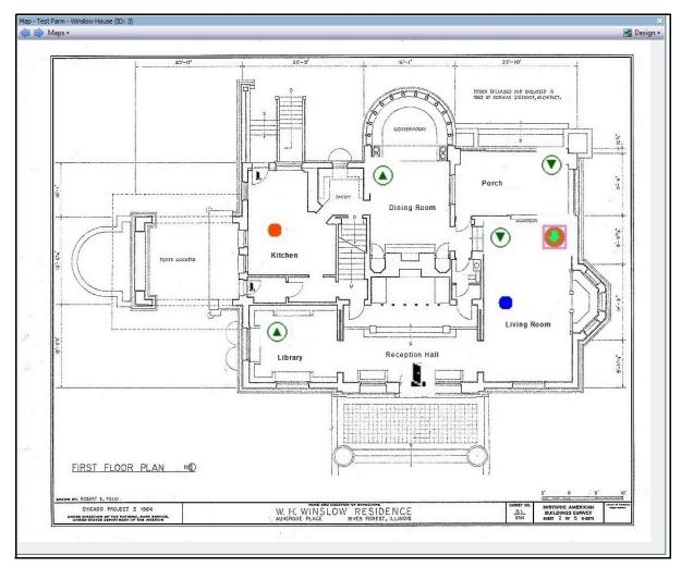
Figure 22. Example of a typical map with camera, PTZ camera, digital I/O, and control access device icons, and rules
