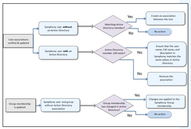
Figure 14. Synchronization Process
