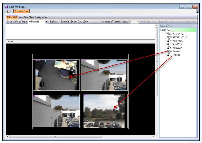
Figure 46. Drag cameras to video wall
